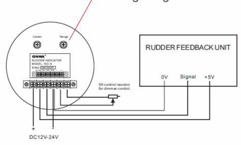
RDI-8 of Rudder Wiring Diagram.
