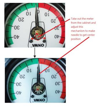
2) Conduct power to Indicators. Place Rudder on zero degree (Mid-ship). Repeatedly adjust the "Center" adjustment on the rear panel of the KRI-80 to ensure all needles are in center position.
