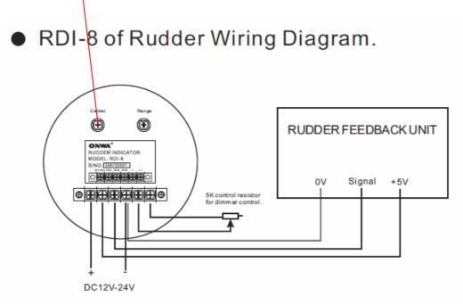
3) Place Rudder to full scale. Adjust the "Range" to read correct Rudder angle indication. For e.g. Full scale of Rudder is 35 degree so you have to adjust every rudder indicator to read 35 degrees.
