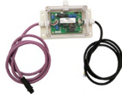
KC-2W N2K (NMEA2000) and NMEA0183 Bidirectional Converter
